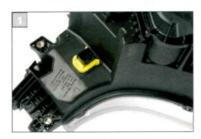
The plug housing is usually positioned on or in the light. Shown here on the headlights of a Mercedes Actros MP4.
