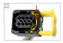
Released retainer – only now can the contacts be unlocked.
