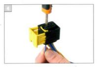
The blades of the tool are pushed in to the stop in the two slots in the desired contact chamber from the contact side. The tool remains in this position and the contact can now be removed by pulling the cable.
